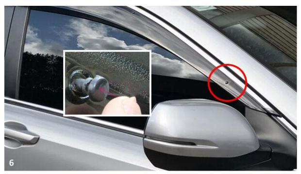
Push the bolt all in, make sure the spread the locker and lock into the nut.
