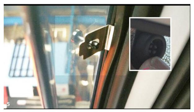
Place the nut from inside, the smooth side face inside the car.
