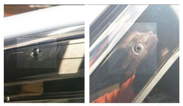
Use heat gun to heat up the tape, then put on the weather shields. Place the locker piece into the hole from outside, then through the clip.
