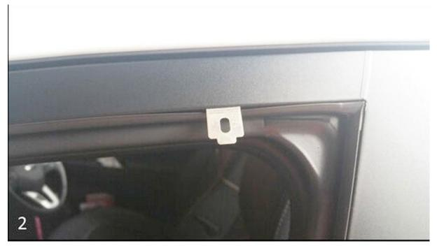
Test-fit the weather shields to check alignment. Mark down the position of the holes, then put clips in the place.
