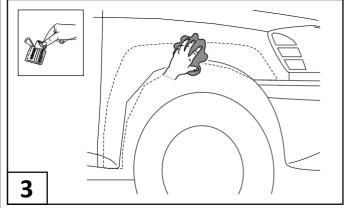
Attach bolts to each Fender Flare using an Allen key and a 1/2" wrench/socket. (wrench/socket and Allen key not supplied)
