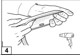
Clean the flares, and then apply the double sided tape to the top edge of the flare. Use heat gun to warn up the tape to make them stick stronger.
