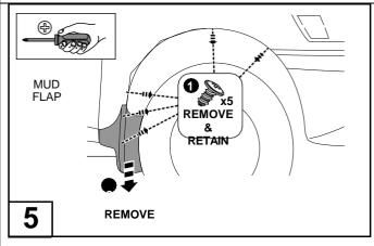
Remove and retain the existing OEM screws from the wheel arch. Remove the mud flaps from the vehicle as shown
