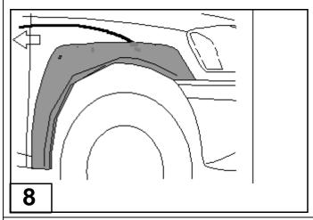
Peel off the double sided tape at last after adjusted position of the flares.
